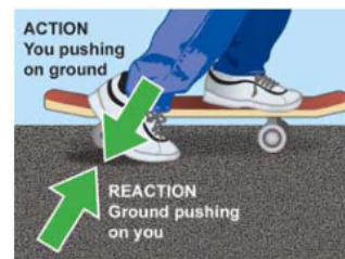
Figure 6.13: You move forward because of the reaction force of the ground on your foot.
