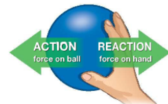
Figure 6.12: Action and reaction forces do not cancel each other out. One force acts on the ball, and the other force acts on the hand.
