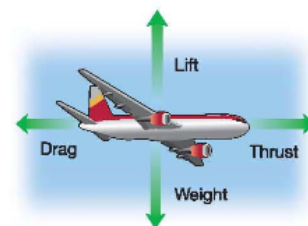
Figure 5.15: Four forces act on a plane as it flies.
