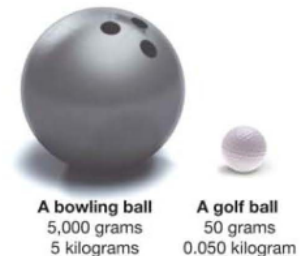
Figure 6.3: The bowling ball has more mass than the golf ball. The bowling ball is harder to move because it has more inertia.
