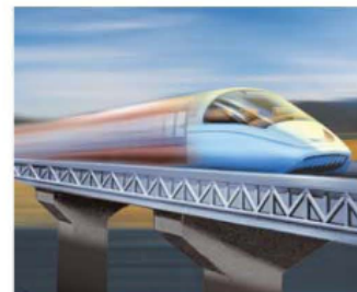
Figure 5.12: With a maglev train, there is no contact between the moving train and the rail—and thus there is little friction.
