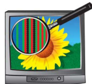
Figure 25.10: A television makes colors using tiny glowing dots of red, green, and blue.
