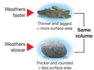
Figure 23.8: A thin, jagged rock has a greater surface area to volume ratio than a thick, rounded rock.
