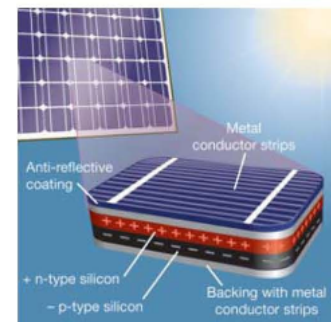
Figure 17.24: A photovoltaic (PV) cell (sometimes called a solar cell) like this one from a solar calculator can convert light energy into a small amount of electrical energy. When light energy strikes the PV cell, electrons from specially treated silicon atoms become free to flow within the electric field set up by the differently charged silicon layers. As you know, a flow of charge like this produces current, which can be directed in a circuit to do work, such as operating a simple calculator.
