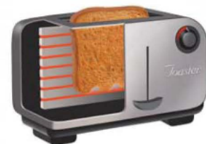
Figure 17.13: A toaster tray is pulled down by an electromagnet while bread is toasting. When the toast is done, current is cut off and the tray pops up. The cutaway shows the heating element—nichrome wires wrapped around a sheet of mica.
