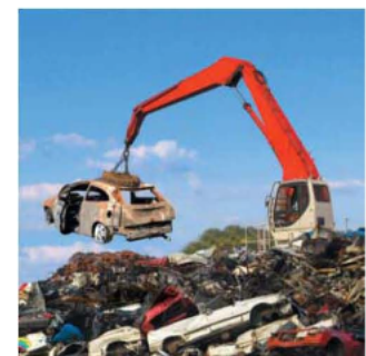
Figure 17.3: Powerful magnets are used to lift cars in a junkyard.
