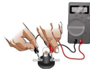
Figure 16.11: A multimeter can be used to measure resistance of a device.
