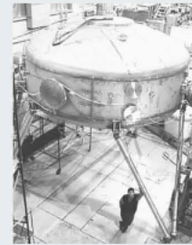
The levitated dipole experiment (LDX) at the Massachusetts Institute of Technology (MIT) uses a superconducting coil to explore fusion technology.
