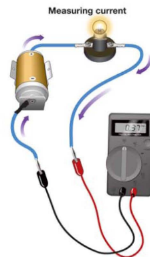
Figure 16.7: Current must pass through the meter when it is being measured.
