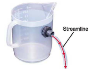
Figure 10.15: Streamlines are imaginary lines drawn to show the flow of a fluid.
