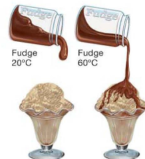
Figure 10.19: Heating fudge topping decreases viscosity so it is much easier to pour.
