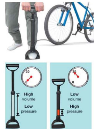
Figure 10.17: Compressing the volume of air to increase the pressure.
