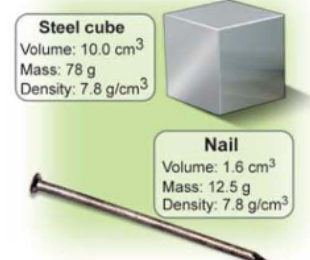
Figure 10.3: The density of a steel nail is the same as the density of a solid cube of steel.
