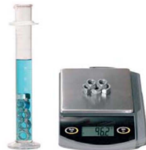
Figure 10.7: A student measures the volume and mass of five steel hex nuts.
