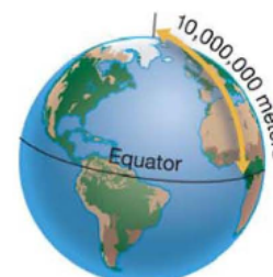
Figure 1.8: In 1791, a meter was defined as 1/10,000,000 of the distance from Earth's North Pole to the equator. Today, a meter is defined more accurately as the distance that light travels in a fraction of a second.
